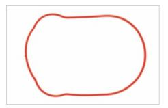
Weather seal for digital readout offers low compression force, yet the best compression set resistance.
